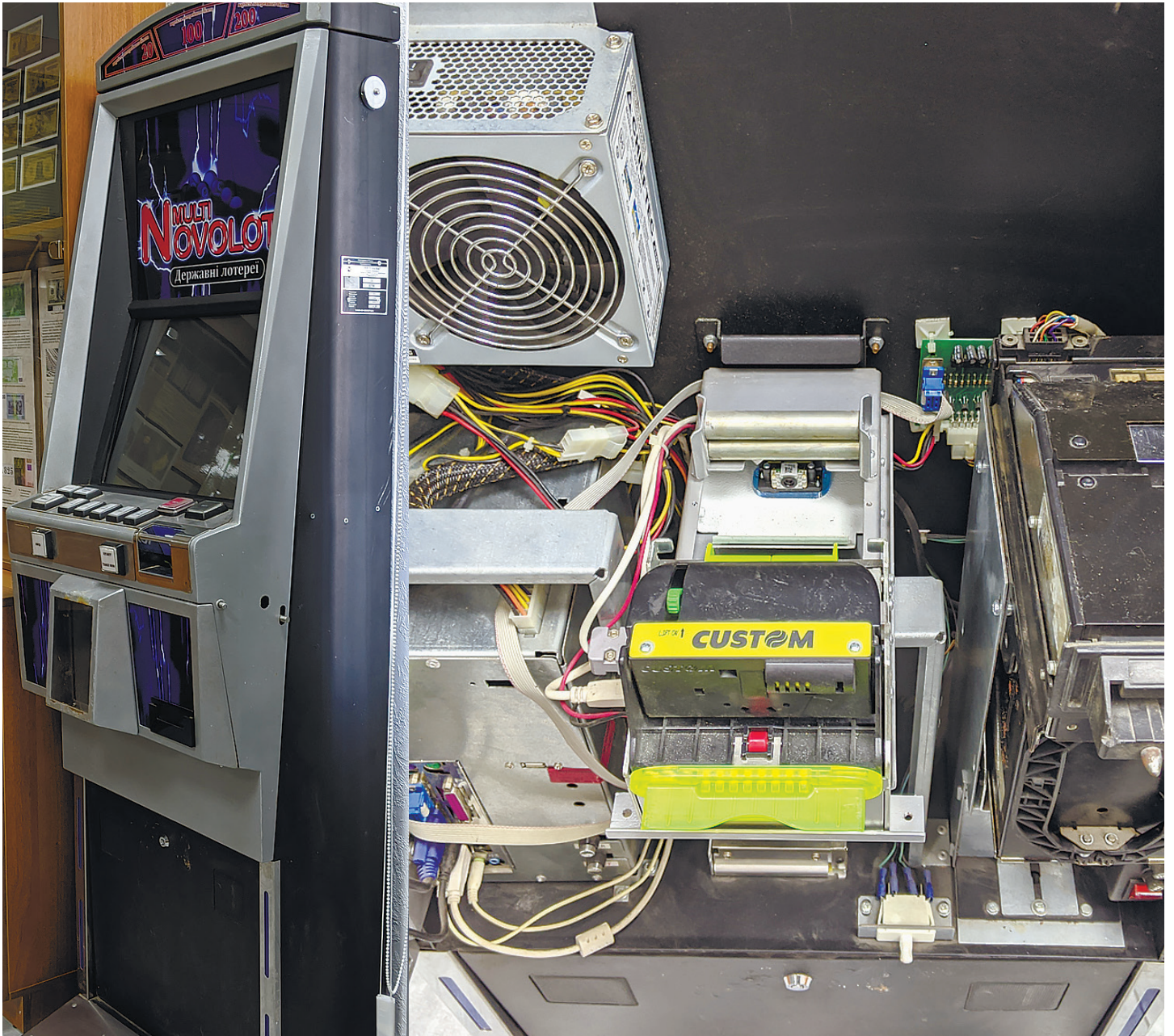
Appearance and internal structure of the slot machine
